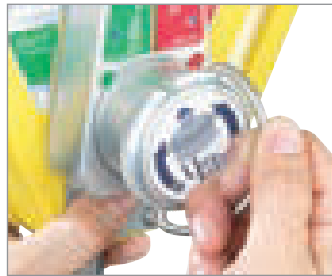
Fall arrest mode Assisted rescue by hand
