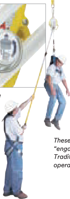
Fall arrest mode Assisted rescue by pole
